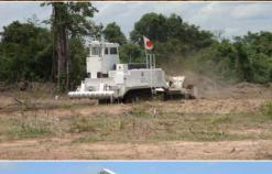
Before 2000, CMAC was very successful working with Japanese manufacturers to design and develop the brush cutters, which were eventually introduced in operations in 2000. These machines have enourmously helped CMAC to speed up demining activities.
